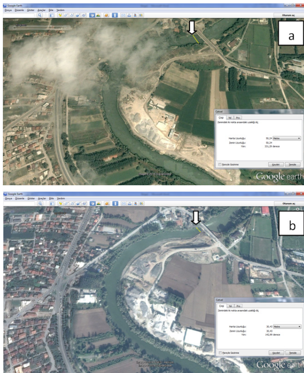
Figure 5. A photograph represents the Sakarya River narrowing process at Historic Sakarya Bridge: (a) Google Earth view in 2003, (b) Google Earth view in 2016
