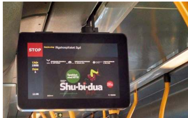
Figure 65: Real time information on zone, line and next stop in a bus (Zone 1)
