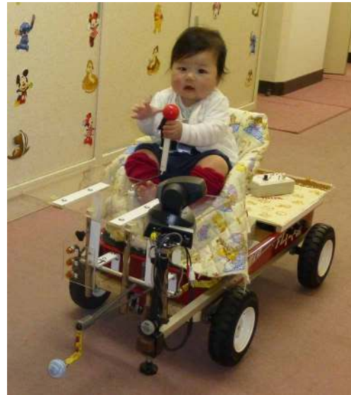
FIGURE 2 | The powered-mobility-device (PMD) used to test the relation between self-produced locomotion and psychological development. Infants can move forward in the PMD by pulling on the brightly colored joystick.
