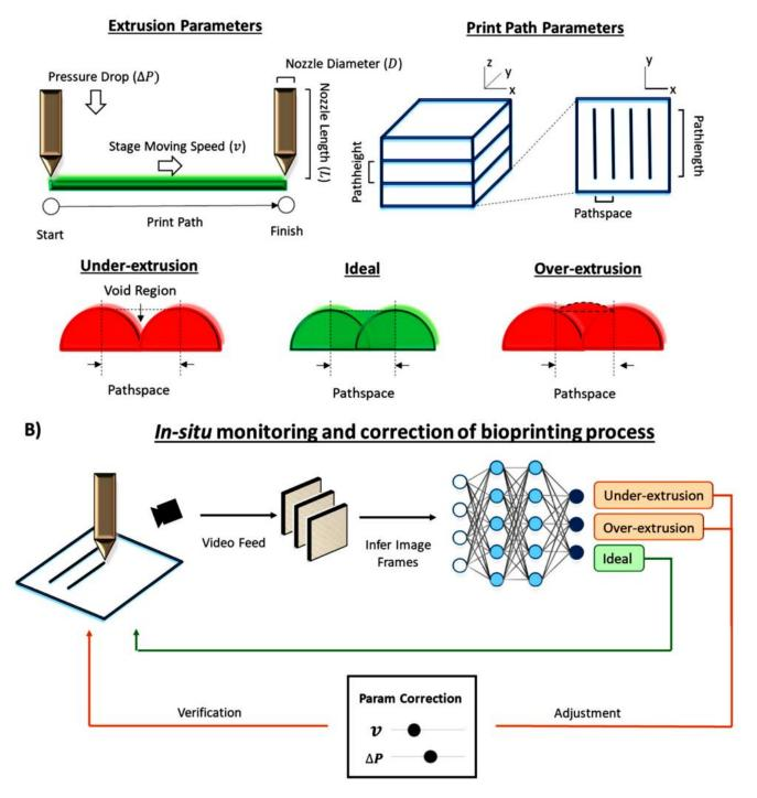
**Figure 9.** (**A**) Three-dimensional bioprinting optimisation processes. (**B**) Computer vision method used for the optimisation and correction of 3D bioprinting using ML approaches. Reprinted with permission from Ref. [12]. 2020, Taylor & Francis Ltd., www.tandfonline.com (accessed on 12 September 2022).
