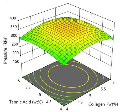
Figure 5. 3D response surface example to optimise the 3D bioprinting pressure.
