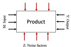
**Figure 4.** P-diagram. A P-diagram is used to classify the variables associated with the product into input energy, signal or user intent (M), noise factors (Z), design parameters (X) and output/key product characteristics, functions, performance, etc. (Y).
