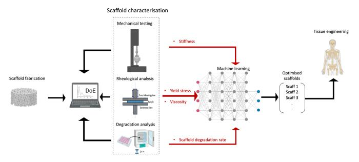
Figure 1. DoE and ML workflow to optimise the material that will be used for the TE applications.
