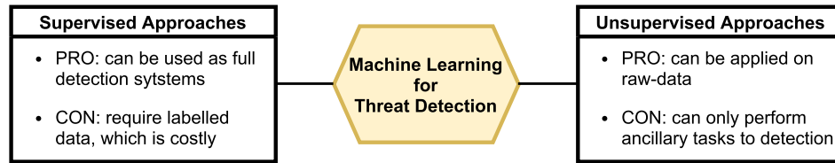
Fig. 3. Pros and cons of supervised and unsupervised ML for cyber threat detection.
