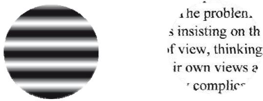
Figure 2.5 Diagrammatic representation of row frequency The lines of letters correspond to the black bars and the spaces between the rows of text correspond to the white bars. This forms the row frequency of 1.2 cpd at 40 cm.
