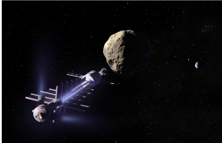
Figure 14 - A So-Called Robotic “Gravity Tractor” Moving an Asteroid into a New Orbit (Courtesy of R. L. Schweickart ND )
