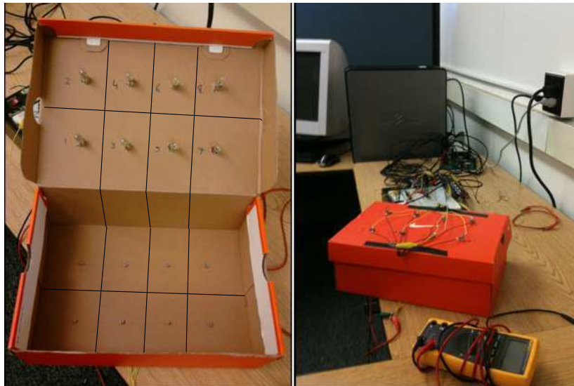
Figure S5. Experimental testbed to model an eight-zones environment. Each zone composed by close lamps and photocells can be divided by “walls” to emulate different cross-illumination conditions. The control strategy is implemented in Simulink through a dSPACE DS1104 DAQ board.
