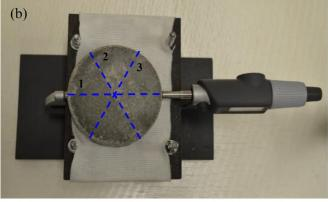
The ultrasonic pulse velocity between the two exposed faces was measured at 500 kHz sampling frequency using a PUNDIT PL-200, while a zero-crossing algorithm was used to calculate the travelling time of the ultrasonic wave. Mass evolution was controlled with a precision balance of ±0.01 g. Surface water of the samples was dried up before weighting.
