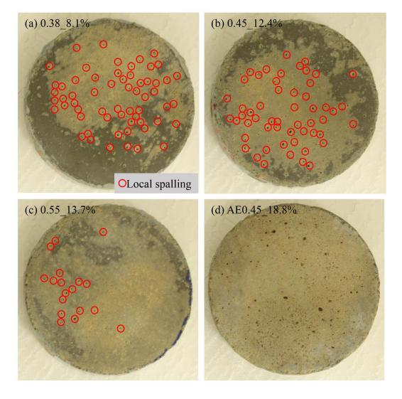
A comparison of the amount of red circles between Figure 4a, 4b and 4c clearly indicates that the physical damage in the form of local spalling increases with the decrease of the porosity of the samples. This observation concurs with the results
