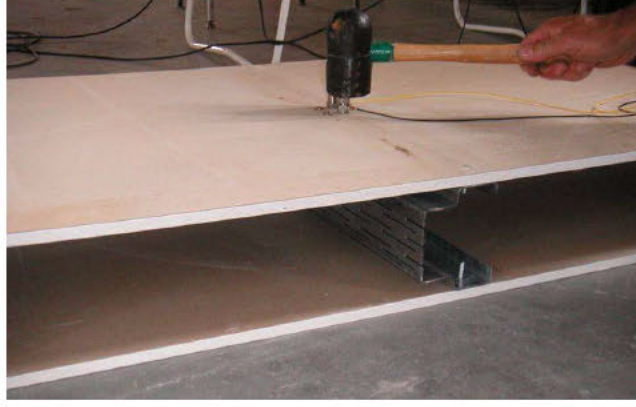
Figure 2: Laboratory tests of the entire package (studs and leaves). The lower leaf is blocked.
