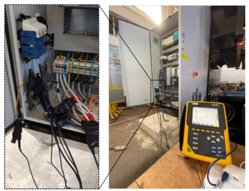
Fig. 2: Cauvin Arnoux C.A 8331 used during the tests
