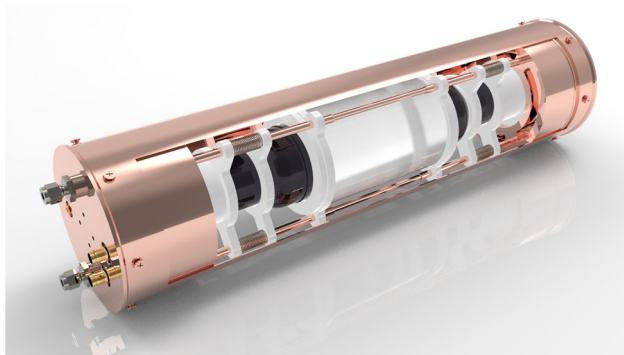
Fig. 1 Rendering of the detector module for the SABRE-PoP phase. The crystal is placed in a copper enclosure; the crystal wrapping is not shown. Two PMTs (black body) are coupled on each end of the crystal. PTFE holders (white) and copper rods keep the crystal and the PMTs in position
