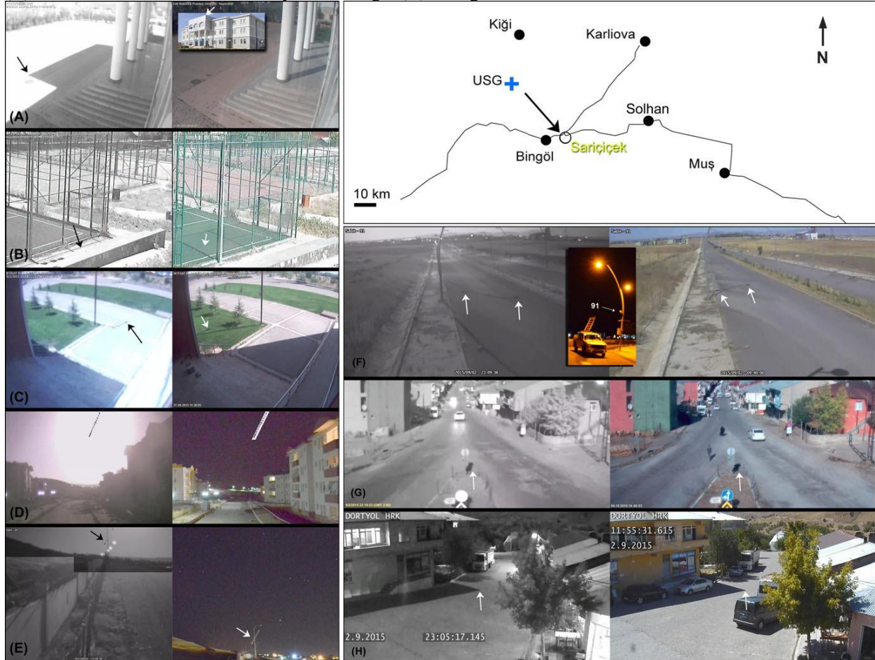
Fig. 1. Example video frames from security camera footage (left) and calibration images (right) used to measure the meteor trajectory and velocity. From top to bottom: (A) Bingöl University rectorate building with the arrows pointing to the tracked feature; (B) Bingöl University soccer court fence; (C) A lamp in front of the Bingöl University campus' faculty of economy cast a shadow on the plaza; (D) Direct imaging by Muş Alparslan University camera #SE3, with dots marking the position of the meteor in subsequent frames, transposed to the star-background calibration image; (E) Muş Alparslan University camera #64, with dots marking the position of the meteor, and the calibration image; (F) Lampposts in view of Muş Alparslan University camera #91 (inset) cast shadows that were tracked on a street; (G) In Karlioiva, shadows were cast by a traffic sign; (H) In Kiği, the roof of a house cast a shadow on the street.
