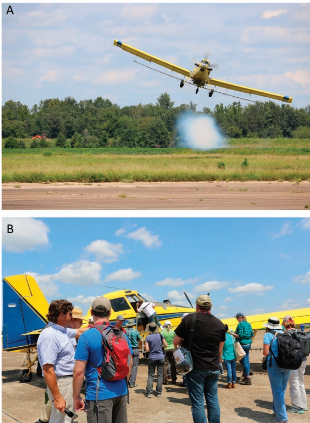
Fig. 2. Tour participants watched a demonstration of how smoke is laid down by aerial applicators to test wind direction to mitigate off-target pesticide drift (top) and to interact closely with a fixed-wing aircraft (bottom) at Provine Helicopter, Inc. in Greenwood, MS (Photo credit: Delta Council).
