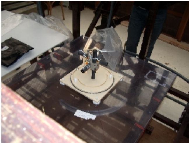
Fig. 10 Tri-axis SCM on a turn-table during tests to determine magnetic axis
