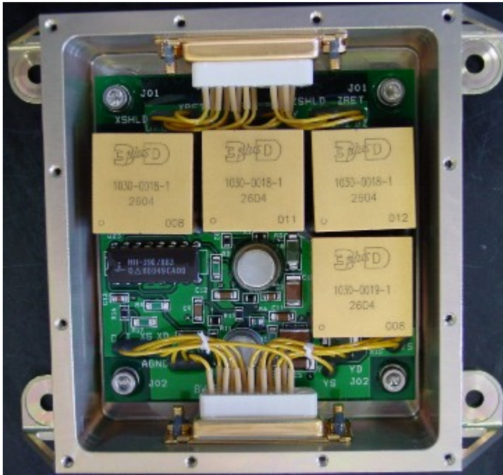
Fig. 6 Preamplifier box. The 3 upper cubes correspond to the 3 antennas preamplifiers, the fourth one is for power regulation. They are manufactured in 3D technology. The electronics for the in-flight calibration is also shown on the PCB. The preamplifier box size is 95 mm x 81 mm (109 with the mounting 'ears') x 30 mm
