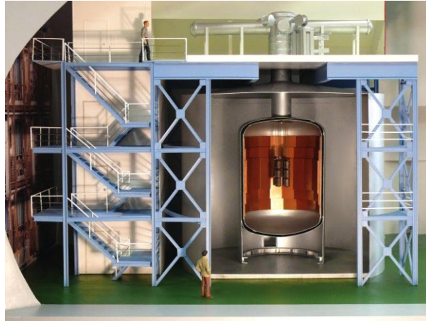
Fig. 25. – Sketch of the GERDA experiment. The germanium arrays can be seen inside the copper cryostat, and this one placed inside the cylindrical water tank.
