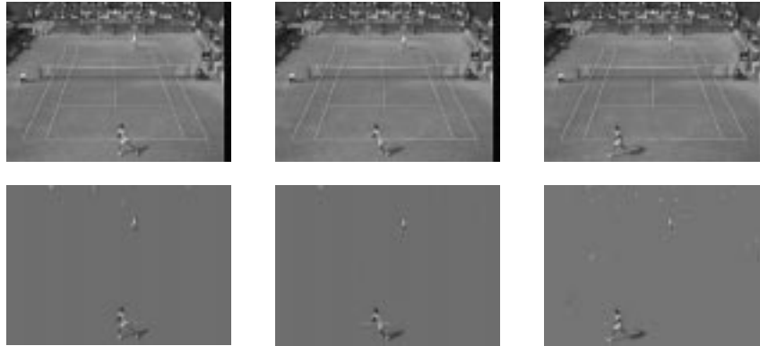
Figure 8: Top row: frames from a 8 bit greyscale movie. Second row: the same frames from which the moving players have been extracted with the help of a scale tree.
