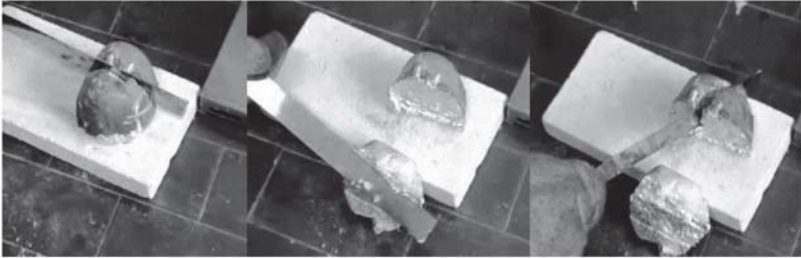
Figure 4. Billet of a semi-solid metal cut with an ordinary knife.
