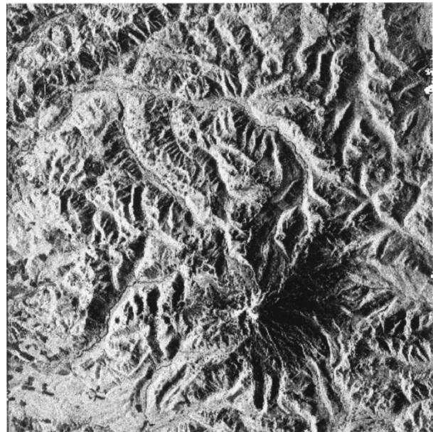
Fig. 6. SIR-C, L -band (horizontally transmitted and vertically received) microwave image of Mt. Rainier, WA. Image was acquired October 1, 1994. A 400 row \times 400 pixel region is displayed. Image courtesy of NASA/JPL.
