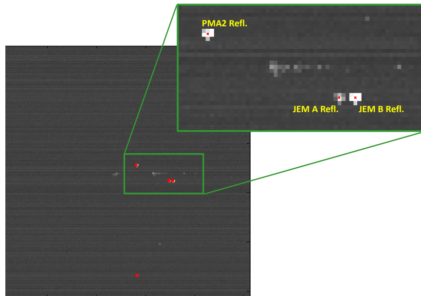
Figure 13. Reflector centroids (denoted by a red \times ) are automatically detected in a VNS image using one of five different methods in the VNSQL Tool. This image was taken during rendezvous with the ISS on flight day 3 of STS-134.
