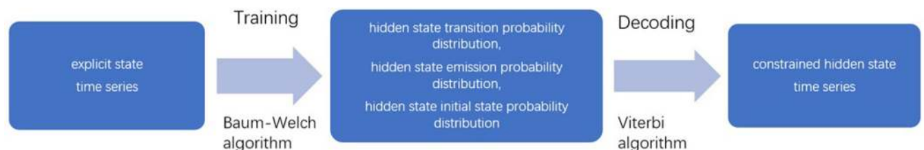
Fig 1. The model training and decoding process of the SDC-HMM. To demonstrate the steps of training and decoding we use the Baum-Welch algorithm and Viterbi algorithm respectively. Firstly, the explicit state time series are trained into the hidden state transition probability distribution, the hidden state emission probability distribution, and the hidden state initial state probability distribution. Then we perform the Viterbi algorithm in decoding these probability distributions into the constrained hidden time series.
