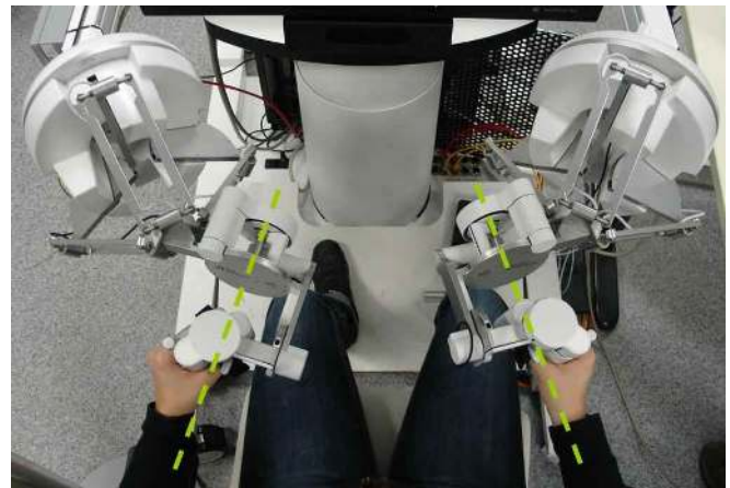
Fig. 5. Bi-manual configuration with axis 4 aligned with the forearm
