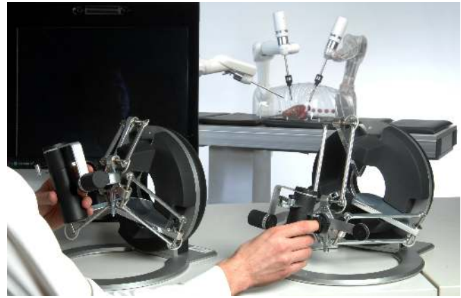
Fig. 2. Foreground: Two omega.7 as master devices; Background: Three Miro robots at an operating table
