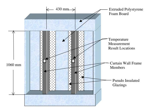
Figure 5. Warm side view of specimen mounting configuration for thermal tests.
