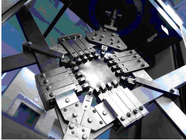
Figure 11. A stretch frame used for equi-biaxial loading of rubber specimens.
