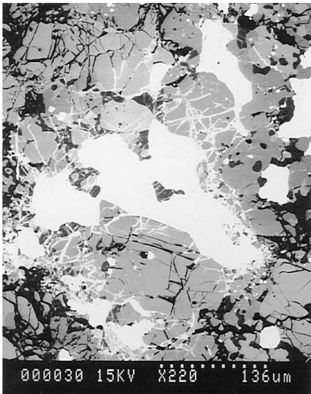
Fig. 4. The H5 ordinary chondrite Épinal in an SEM backscatter image. The large white areas are Fe, Ni grains; the dark lines are a series of microcracks, which account for the measured porosity. Note the microcracks partially filled with white material; this is interpreted as the oxidation product of terrestrial oxygen reacting with the meteoritic iron.
