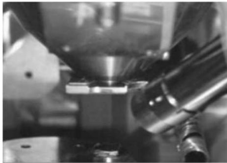
Figure 5: The position of secondary, back-scattered, and X-ray detectors [55].
