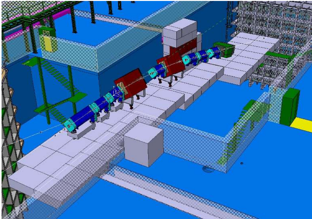
Figure 6.2: Layout of the quadrupole and dipole magnets in the H4 beamline extension. The secondary target (not shown) is upstream of the first quadrupole magnet on the left side of the Figure. Vacuum beam pipe and beam instrumentations are also not shown. (Courtesy of V. Clerc, CERN).
