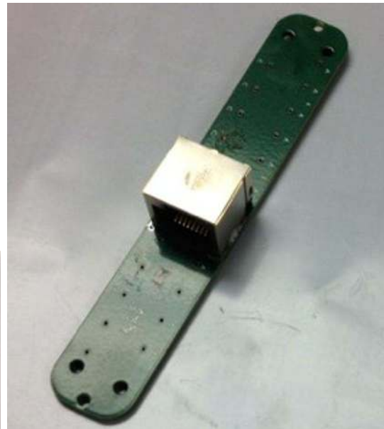
Figure 2.54: Photograph of a SiPM mounting board with the full complement of 12 SiPMs installed on the board (left), and with the RJ-45 connector for the cable (right).
