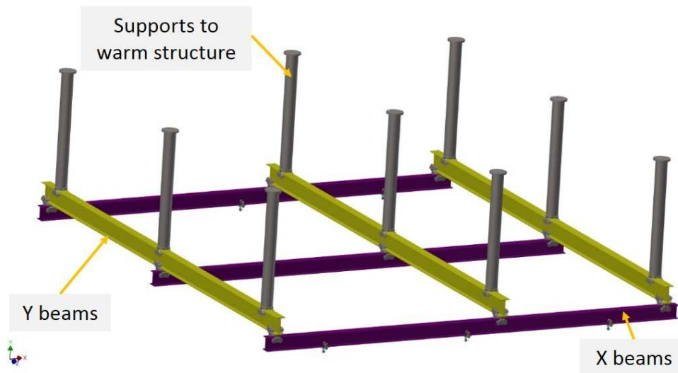
Figure 2.65: Detector support system
