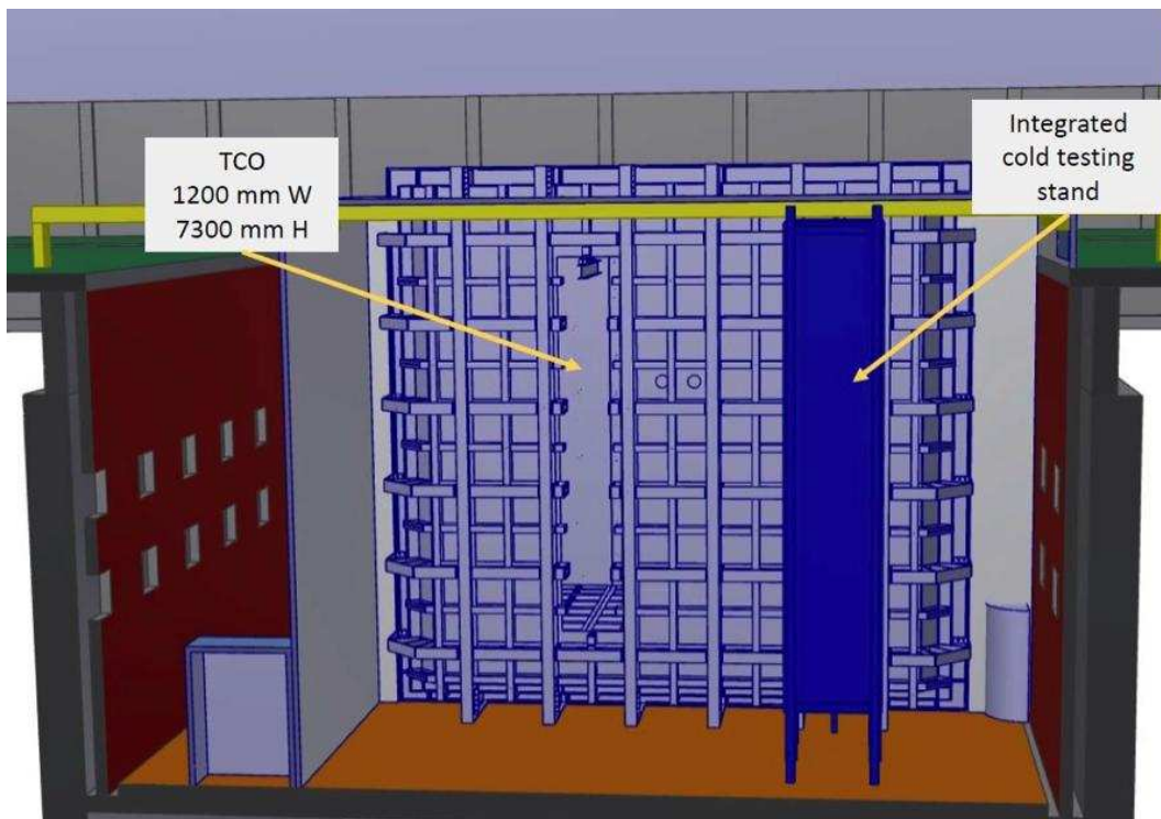
Figure 3.3: Elevation section view of the cryostat
