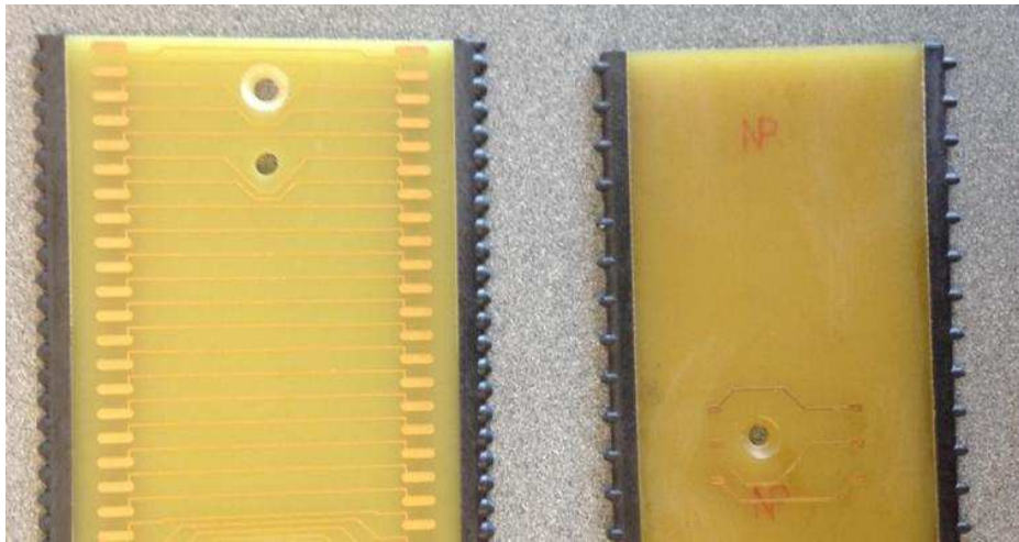
Figure 2.9: Boards with injection molded tooth strips glued on. The left shows an end board with teeth for fixing the position of the longitudinal wires. The teeth there form small notches. The right is a side board for fixing the position of the angled wires where the wires are angled around a pin. (These boards are prototype test pieces and are not used in the production APAs.)
