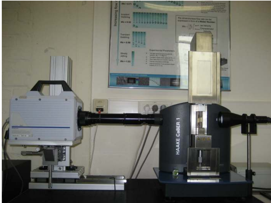
Figure 1: Experimental set up for the CaBER.
