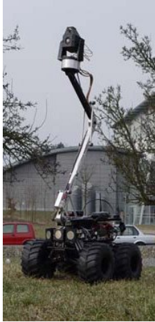
Fig. 2. The Outdoor MERLIN with the deployed standard mast configuration, elevating the camera for monitoring purposes to 1 m height for better panoramic view.
