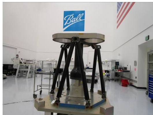
Figure 9: IXPE MMSS Deck Attached to Center-tube on Spacecraft Top Deck and Bipods Assemblies
