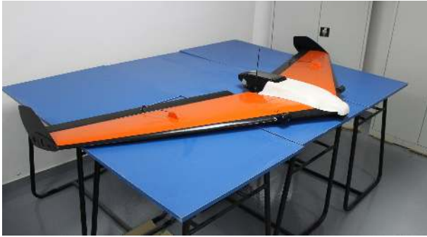
Figure 3. The 2.5 m wingspan flying-wing UAV developed in parallel with SWING.
