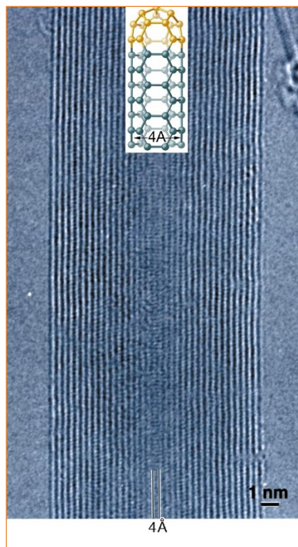
Figure 1 High-resolution electron microscope image of a 4 Å tubule (side walls are marked by lines) confined inside an 18-shell carbon nanotube. Dark lines correspond to the side walls of the single-wall shells. The blurring towards the centre is due to the smaller number of atoms in the smaller tubules. Inset, model for the formation and growth of a [3,3] armchair tubule of 4 Å diameter. Half of the C 20 dodecahedron (yellow) serves as a nucleus and further growth into the tubule is realized by adding carbon atoms (blue).
