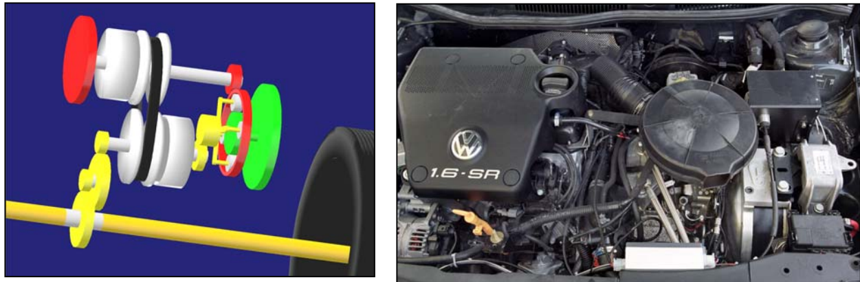
Figure 4: Zero Inertia (ZI) Powertrain: CVT with powersplit-rotor (by Drivetrain Innovations)
