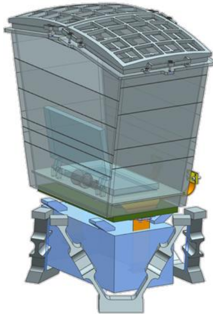
Figure 1. A stripped-down mechanical drawing of the SXI, showing the optics at the top of the instrument that are used to focus the soft X-rays onto the focal plane which is positioned below a shielding door (shown open in this configuration). The CCDs in the focal plane are electrically connected to the Front End Electronics (FEE) that is contained in the blue box. A thermal radiator and optical baffle are not shown here. The instrument interfaces with SMILE’s Payload Module via the tripod design at the base.
