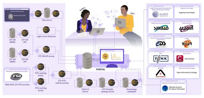
Figure 9. Diagram of the service infrastructure. Dashed rectangles represent individual services, circles are web modules and complimentary scripts, cylinders are database management systems, and the display is the Portal module. Parallelograms are external services used by the Viewer. Lines show data flow, double circles mark data receivers. Arrows show data exchange between modules of a single service.
