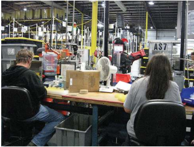
Figure 5. Two operators working near the robot. The vantage point of the operators makes it difficult to monitor the robot's status. Additionally, the tasks the operators are completing requires their visual attention.
