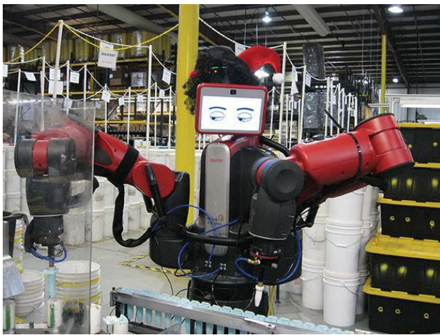
Figure 2. Examples of a collaborative robot at work packaging medicine cups at Company 1 (top) and moving plastic tubes at Company 2 (bottom).
