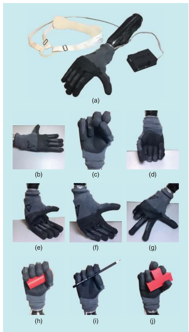
Figure 4. (a) The SHPH prototype adopted for the C-PAPR and its main components: the hand, the socket, the body power harness, and the battery pack. The main hand postures available to the user include (b) flat hand, (c) grasp closure, (d) and fist. (e)–(g) The soft behavior of the SoftHand and its robustness in several interactions with the environment. (h)–(j) The main grasping capabilities of the hand, highlighting the intrinsic adaptability to object shape.
