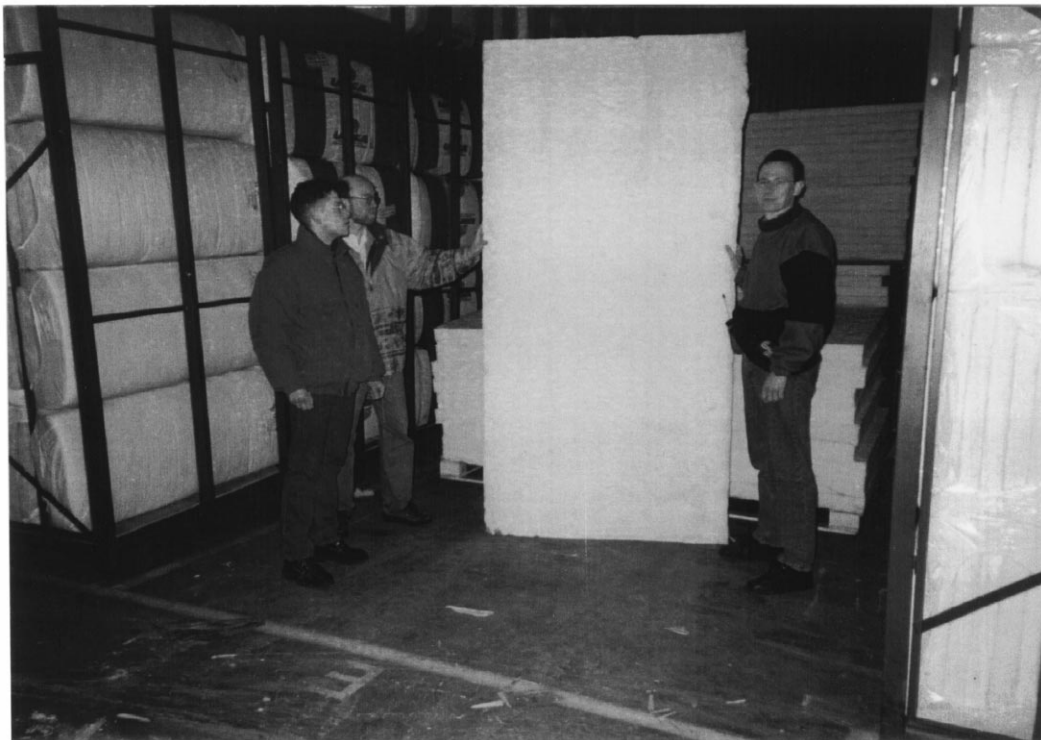
Figure 6. Glass fiber insulation mats fabricated on an industrial scale with the new binder.
