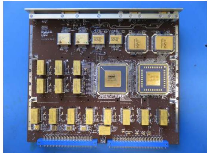
Fig. 17. Processor Board in the EUI CEB. At the bottom of the board there are gigabytes of SDRAM for the One-Hour-Queue (OHQ) seen as eight blocks, and at the very bottom in the middle is the flash memory. The Spacecraft Output Buffer (SOB) is located in the middle left as six blocks. The Processor Board FPGA is at the centre with the UT699 CPU to the right. The two components to the top left are the MRAM. The next four components (two small, two large) on the top right are the CPU SRAM.
