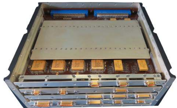
Fig. 2. CEB of EUI with the top and front panels removed.
