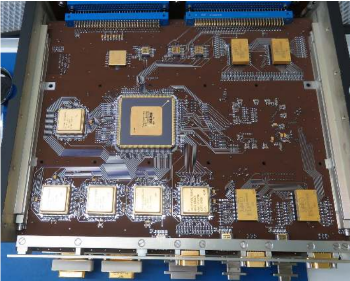
Fig. 18. EUI CEB Compression Board. The Compression Board FPGA is the large integrated circuit near the centre. The block on the middle left together with the first three of the bottom row are the compression SRAM. The WICOM is the fourth block of the bottom row. On the top right and bottom right there are four SDRAMs for the WICOM.
