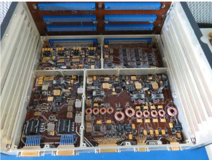
Fig. 20. EUI CEB power supply unit. The top left are the voltage regulators for internal supplies, the top right is the housekeeping filtering and conditioning, the bottom left is the CEB PSU, and the bottom right are the camera PSUs.
