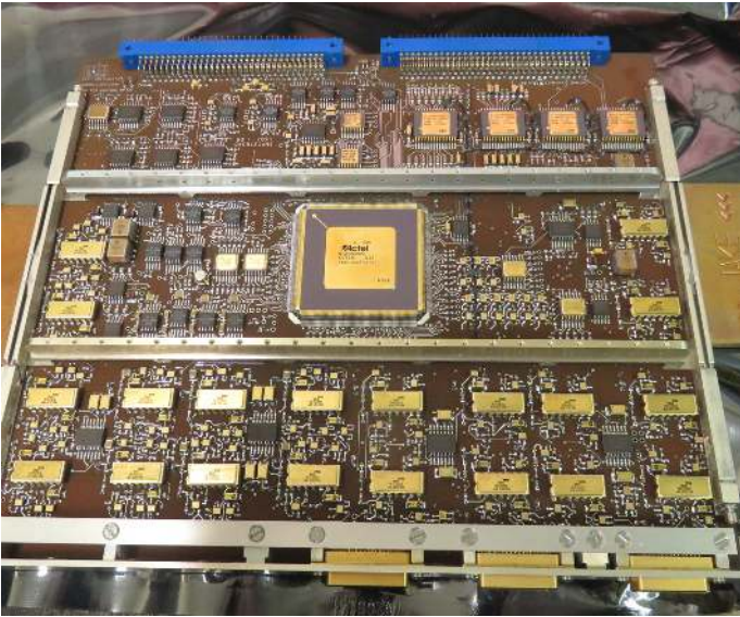
Fig. 19. EUI CEB auxiliary board. The AUX board FPGA is at the centre. The bottom third of the board contains the motor drive circuitry. Housekeeping is digitized in the top part of the board.
