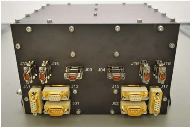
Fig. 27. SWA-DPU flight model hardware.
