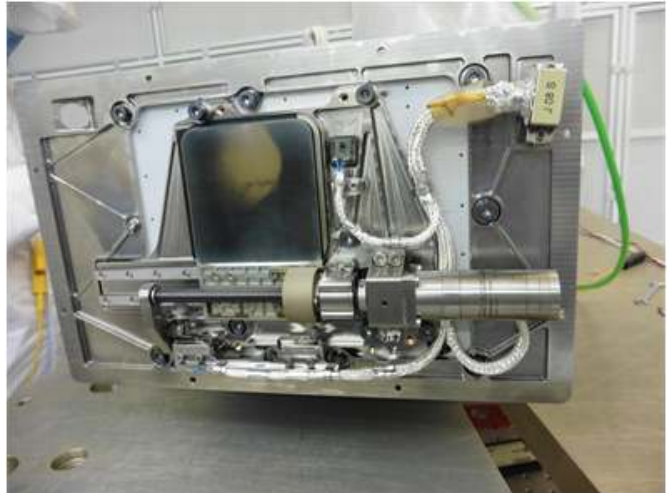
Fig. 10. Door Mechanism. The drawing on the left highlights its components, the picture on the right shows the assembled flight model.
