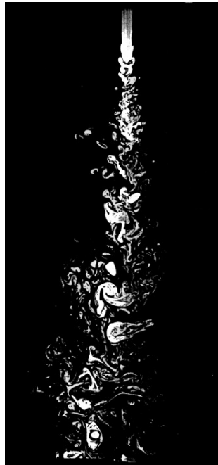
Figure 3: Turbulence as observed in a turbulent water jet (Van Dyke, 1982) reported in the book by Frisch (1995) (photograph by P. Dimotakis, R. Lye, and D. Papantoniou).
