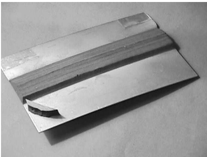
Figure 4. An SSF sample of OFTi on aluminum substrate (a cross-section of sample on left) powder and driving the SSF nozzle. The saddle bed of the lathe, equipped with a pneumatic cylinder, was used to translate the nozzle within the debris recovery cabinet.
