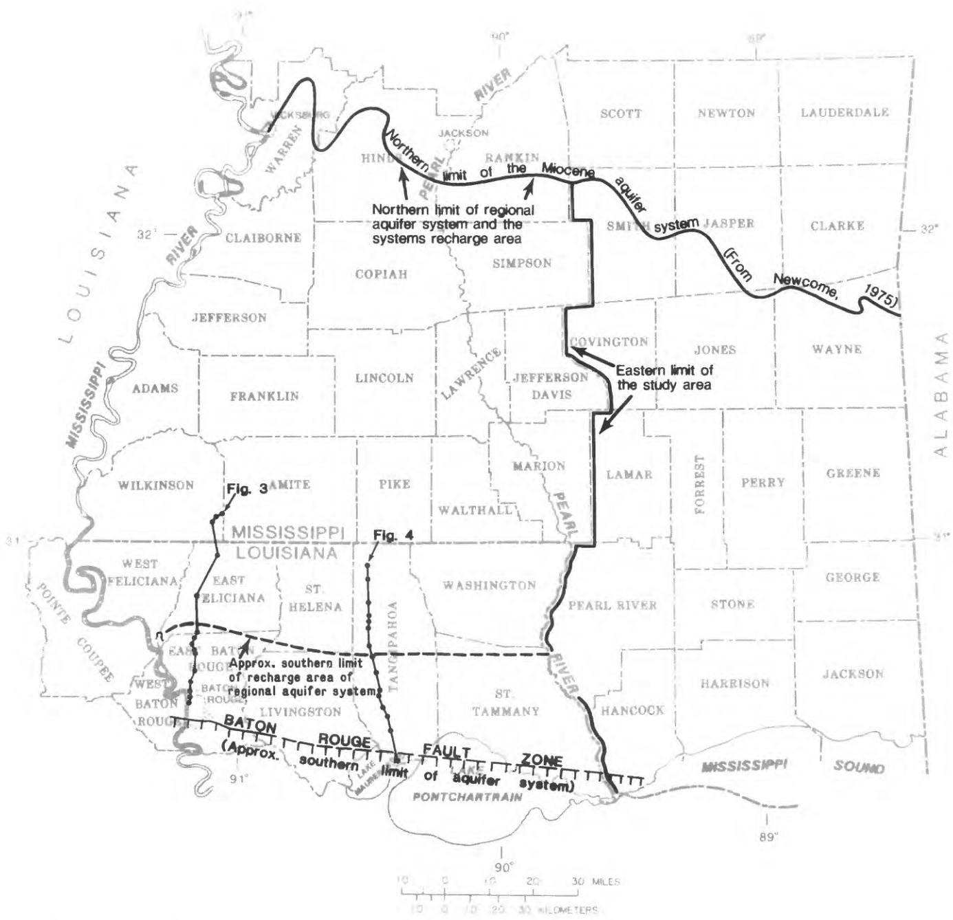
Figure 2.--The extent and recharge area of the aquifer system and locations of detailed geohydrologic sections.
