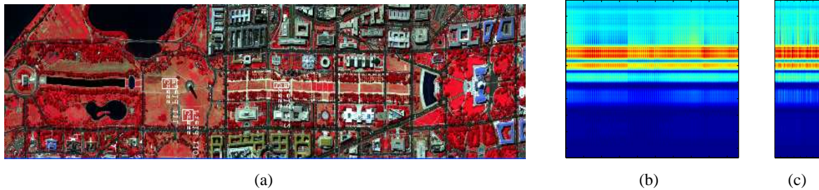
Fig. 11. (a) Simulated color IR view of an airborne hyperspectral data over the Washington DC Mall [37]. (b) Ground-truth pixel spectrum of grass pixels that are outlined with the white rectangles in (a). (c) Synthesized data spectrum using the Gaussian distribution.
