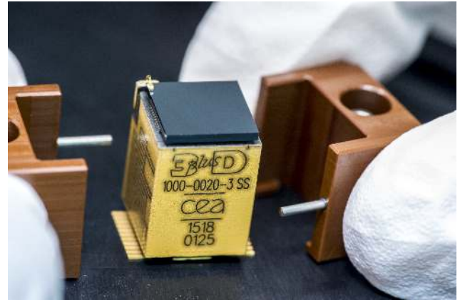
Fig. 13. View of Caliste-SO with a crystal mounted on the top. The picture is taken during the process of removal of the protective holder used for performance tests and transportation. The Caliste-SO body dimensions are about 11 \times 12 \times 15\ \text{mm} high. Credit: L. Godart/CEA.
