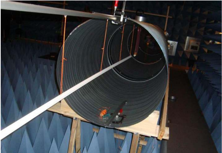
Fig. 32 Test setup for tests of FM17 BEB + boom cable + preamp in IRFU EMC chamber
