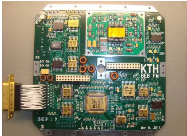
Fig. 14 Photo of FM17 BEB CP board (with EMC shield removed)
