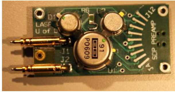
Fig. 17 Photo of FM30 preamp board. The boom cable attaches to the right
