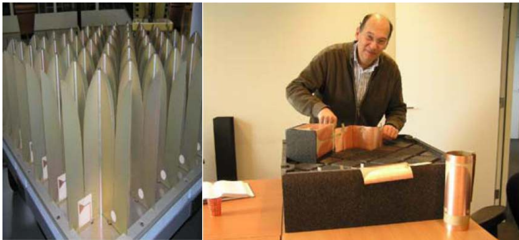
Figure 8: Left – Prototype aperture array elements for EMBRACE. Right – experimentation with highly manufacturable elements for aperture arrays, in this instance utilizing a printing process for depositing the metallic elements on thin plastic film.
