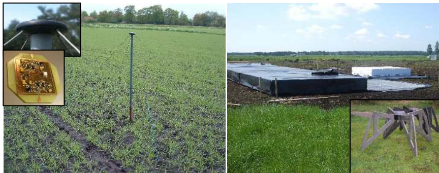
Figure 6: An example of elements of sparse aperture arrays, the LOFAR antennas (ASTRON, The Netherlands). On the left is a polarization pair of “droopy dipoles” that operate from 30-80 MHz. The inset shows the low noise amplifier hub. On the right is a “tile” of LOFAR high-band antennas, with the individual elements shown in the inset.
