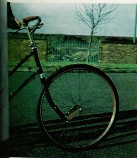
"UNRIDABLE" BICYCLES. David Jones is seen here with three of his experimental machines, two of which turned out to be rideable after all. At top of this page is URB I, with its extra counter-rotating front wheel that tests the gyroscopic theories of bicycle stability. At left is URB III, whose reversed front forks give it great stability when pushed and released riderless. URB IV (immediately above) has its front wheel mounted ahead of the usual position and comes nearest to being "unridable." —FIG. 1
