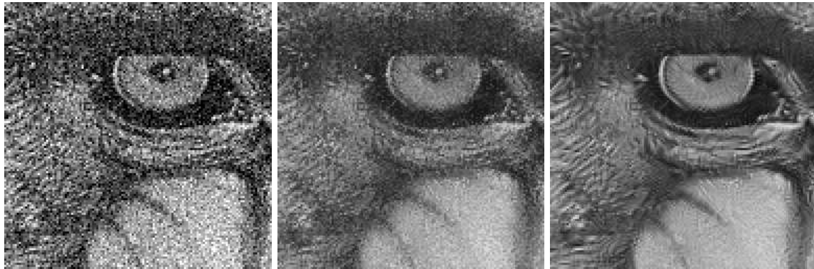
Fig. 7. Comparison of the linear regression neighborhood filter and the linear regression NL-means. Left: Noisy image. Middle: Linear regression neighborhood filtered image. Right: Linear regression NL-means filtered image.
